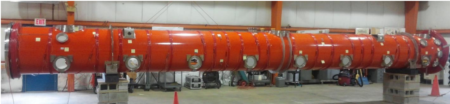
Helmholtz coils wound onto vessel directly
